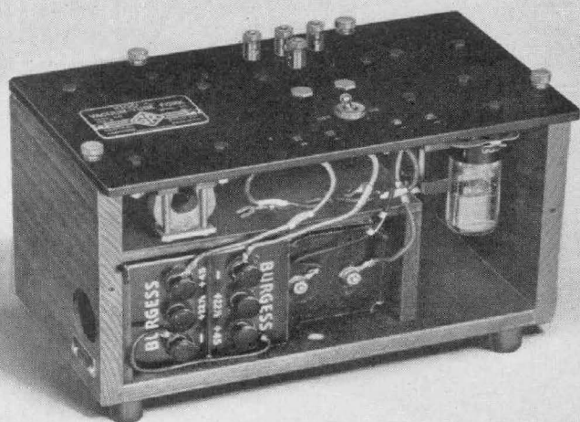
FIGURE 3. Views showing the power-supply compartment. Left, battery supply and, right, a-c power supply.
